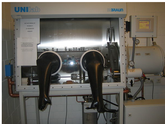
Gloveboxes are often filled with argon, which recirculates over scrubbers to maintain an oxygen-, nitrogen-, and moisture-free atmosphere
