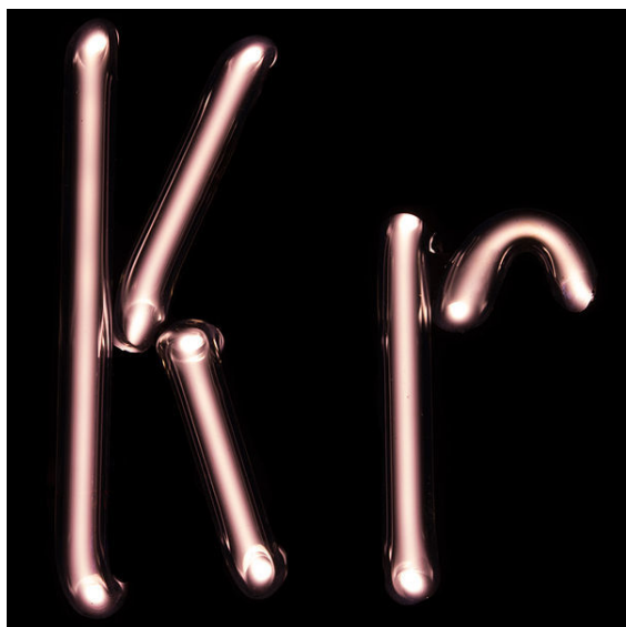
Krypton gas discharge tube
