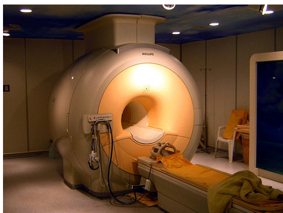
Liquid helium is used to cool the superconducting magnets in modern MRI scanners
