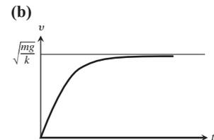
(c)  $v_{\text{terminal}} = \sqrt{\frac{160}{0.005}} = 178.9 \text{ ft/seg} = 122 \text{ mph}$
