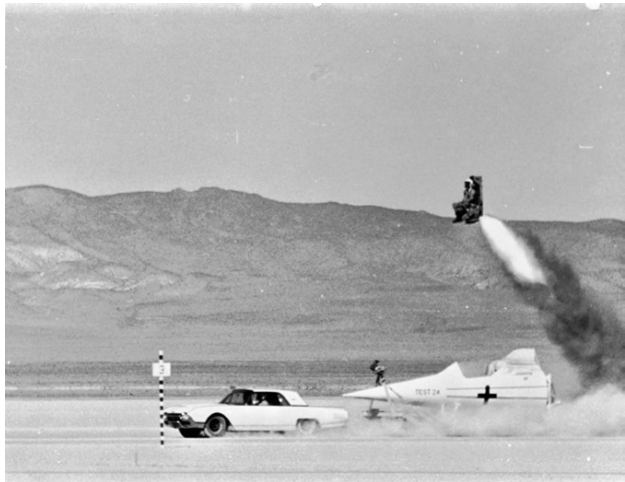
A-12 ejection-seat test on Groom Lake's dry lake bed. (Collection of Roadrunners Internationale/CIA)
