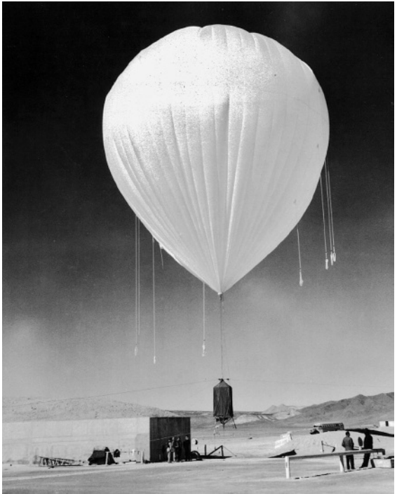
The black device attached to this balloon in Area 9 of the Nevada Test Site is a 74-kiloton atomic bomb code-named Hood, the largest atmospheric nuclear weapon ever exploded in the United States. Standing on a ladder minutes before this photograph was taken on July 5, 1957, Al O'Donnell put the final touches on the bomb's firing
