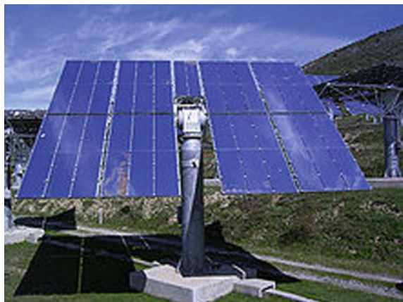
Fig. 2.12 View of a heliostat mirror
