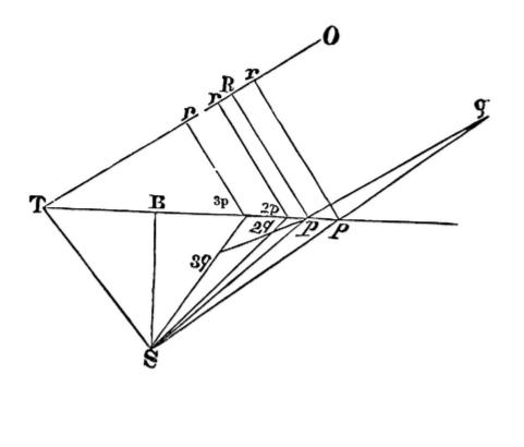
*rp* meeting TP in *p*. Then through the point S*p* draw the line S*q* equal to  $\frac{M^2 \times N}{Or^2}$ . In like manner draw three or more right lines S2*q*, S3*q*, &c., and a regular line *q*2*q*3*q*, drawn through all the points *q*2*q*3*q*, &c., will cut the right line TP in the point P, from which the perpendicular PR is to be let fall. Q.E.F.
