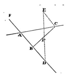
From the given point P suppose any right line PD to be drawn to either of the right lines given, as AB; and produce the same towards AC, the other given right line, as far as E, so as PE may be to PD in the given proportion. Let EC be parallel to AD. Draw CPB, and PC will be to PB as PE to PD. Q.E.F.
