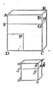
Let the fluid be supposed to be included in a cubic space ACE, and then to be reduced by compression into a lesser cubic space *ace*; and the distances of the particles retaining a like situation with respect to each other in both the spaces, will be as the sides AB, *ab* of the cubes; and the densities of the mediums will be reciprocally as the containing spaces AB<sup>3</sup>, *ab*<sup>3</sup>. In the plane side of the greater cube ABCD take the square DP
