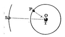
Therefore the perturbation is least when the common centre of the three bodies is at rest; that is, when the innermost and greatest body T is attracted according to the same law as the rest are; and is always greatest when the common centre of the three, by the diminution of the motion of the body T, begins to be moved, and is more and more agitated.
