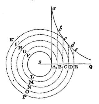
Let AFL be a cylinder turning uniformly about the axis S, and let the concentric circles BGM, CHN, DIO, EKP, &c., divide the fluid into innumerable concentric cylindric solid orbs of the same thickness. Then, because the fluid is homogeneous, the impressions which the contiguous
