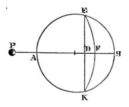
Let the body P placed in the axis ADB of the segment EBK be attracted by that segment. About the centre P, with the interval PE, let the spherical superficies EFK be described; and let it divide the segment into two parts EBKFE and EFKDE. Find the force of the first of those parts by Prop. LXXXI, and the force of the latter part by Prop. LXXXIII, and the sum of the forces will be the force of the whole segment EBKDE. Q.E.I.
