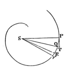
Let that spiral be PQR. From the velocity, with which the body goes over the very small arc PQ, the time will be given; and from the altitude TQ, which is as the centripetal force, and the square of the time, that force will be given. Then from the difference RS*r* of the areas PSQ and QSR described in equal particles of time, the retardation of the body will be given; and from the retardation will be found the resisting force and density of the medium.
