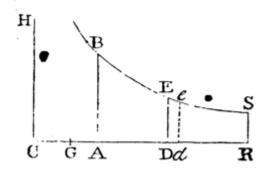
In the asymptote CD let there be given the point R, and, erecting the perpendicular RS meeting the hyperbola in S, let the space described be expounded by the hyperbolic area RSED; and the velocity will be as the length GD, which, together with the given line CG, composes a length CD decreasing in a geometrical progression, while the space RSED increases in an arithmetical progression.
