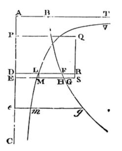
Suppose the body E to fall from any place A in the right line ADEC; and from its place E imagine a perpendicular EG always erected proportional to the centripetal force in that place tending to the centre C; and let BFG be a curve line, the locus of the point G. And in the beginning of the motion suppose EG to coincide with the perpendicular AB; and the velocity of the body in any place E will be as a right line whose square is equal to the curvilinear area ABGE. Q.E.I.
