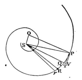
Cor. 5. And because at equal distances from the centre the velocity is the same in the spiral PQR as it is in the right line SP, and the length of the spiral is to the length of the right line PS in a given ratio, namely, in the ratio of OP to OS; the time of the descent in the spiral will be to the time of the descent in the right line SP in the same given ratio, and therefore given.
