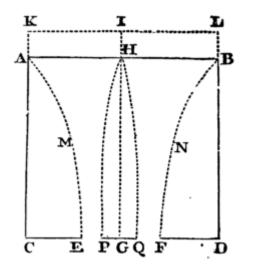
Cor. 7. If in the middle of the hole EF there be placed the little circle PQ described about the centre G, and parallel to the horizon, the weight of water which that little circle sustains is greater than the weight of a third part of a cylinder of water whose base is that little circle and its height GH. For let ABNFEM be the cataract or column of falling water whose
