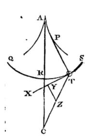
Let the body T oscillate in any curve line STRQ, whose axis is AR passing through the centre of force C. Draw TX touching that curve in any place of the body T, and in that tangent TX take TY equal to the arc TR. The length of that arc is known from the common methods used for the quadratures of figures. From the point Y draw the right line YZ perpendicular to the tangent. Draw CT meeting that perpendicular in Z, and the centripetal force will be proportional to the right line TZ. Q.E.I.
