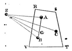
Let the particles A, B, of the body RSTV attract any corpuscle Z with forces which, supposing the particles to be equal between themselves, are as the distances AZ, BZ; but, if they are supposed unequal, are as those particles and their distances AZ, BZ, conjunctly, or (if I may so speak) as those particles drawn into their distances AZ, BZ respectively. And let those forces be expressed by the contents under  $A \times AZ$ , and
