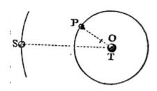
For the attractions of the body S towards T and P compose its absolute attraction, which is more directed towards O, the common centre of gravity of the bodies T and P, than it is to the greatest body T; and which is more in a reciprocal proportion to the square of the distance SO, than it is to the square of the distance ST; as will easily appear by a little consideration.
