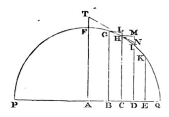
In the same manner that the density of the medium comes out to be as  $\frac{S \times AC}{R \times HT}$ , in Cor. 1, if the resistance is put as any power V<sup>n</sup> of the velocity V, the density of the medium will come out to be as  $\frac{S}{R\frac{4-n}{2}} \times \left(\frac{AC}{HT}\right)^{n-1}$
