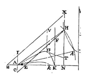
Therefore if a body projected from the place A, in the direction of the right line AH, describes the hyperbola AGK and AH produced meets the asymptote NX in H, and AI drawn parallel to it meets the other asymptote MX in I; the density of the medium in A will be reciprocally as
