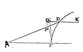
Cor. 2. If a body lighting on any superficies CD in the direction of a right line AD, drawn according to any law, should emerge in the direction of another right line DK; and from the point C there be drawn curve lines CP, CQ, always perpendicular to AD, DK; the increments of the lines PD, QD, and therefore the lines themselves PD, QD, generated by those increments, will be as the sines of incidence and emergence to each other, and*è contra*.
