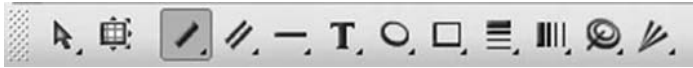
FIGURE 8.9 The toolbar contains all the drawing tools, including the trendline, which is the third from the left.
