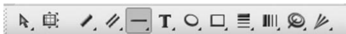
FIGURE 11.6 The horizontal tool is the fifth selection on the toolbar, located between the channel and text tools.
