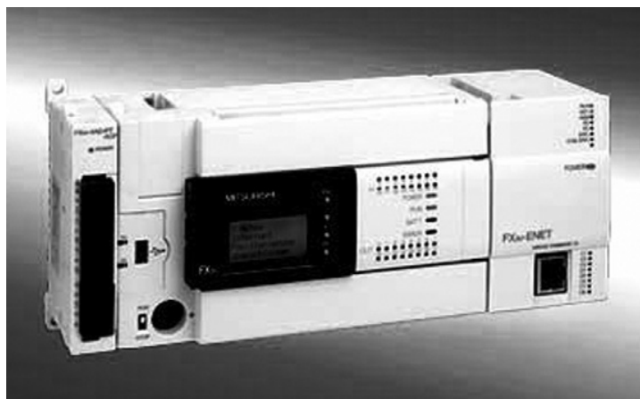
Figure 1.13: Mitsubishi Compact PLC: MELSEC FX3U. (By permission of Mitsubishi Electric Europe.)
