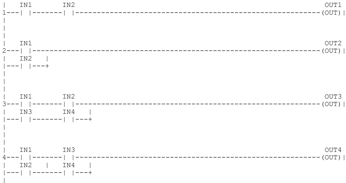
Figure 3-8 - PLC Program with AND-OR and OR-AND Added
