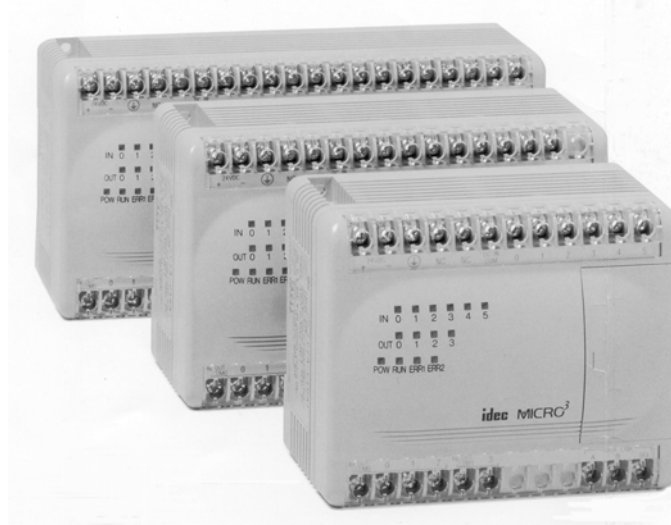
Figure 2-2 - Shoebox-Style PLCs (IDEC Corp.)
